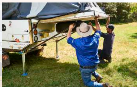
Attach the clevis end of the bed support to the bottom of the lid
