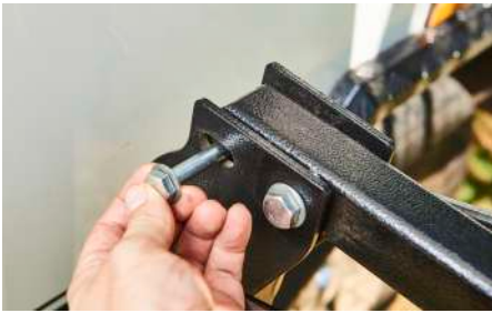
Remove the locking bolts on the other side of the trailer
