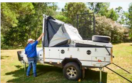
It's essential to carefully lower the lid, and do not let it drop onto the trailer, as damage may occur
