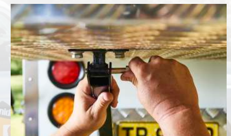
Ensure the pin goes through both the support pole and the loop on the lid
