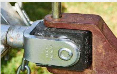
Now remove your Treg hitch pin completely
