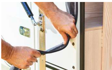
Attach the press studs while the canvas is still slack
