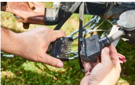
Disconnect your trailer plug & any other elec. connections to the trailer
