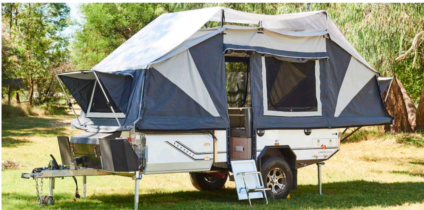
Take your time extending the bows, and make sure that both the left and right sides are extended evenly
