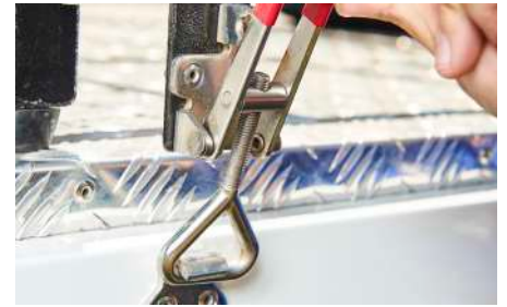
Release the over-centre catches
