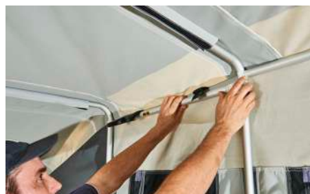
Spreader bars keep the bows where they need to be
