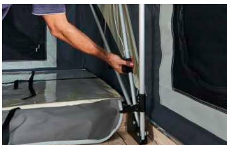
Take your time extending the bows, and make sure that both the left and right sides are extended evenly
