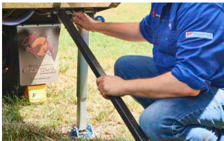
The solid end (without the clevis) attaches to the trailer
